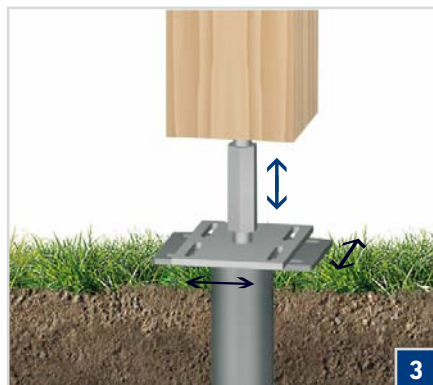
3 Place the post anchor (with post) onto the flange plate and align it.
