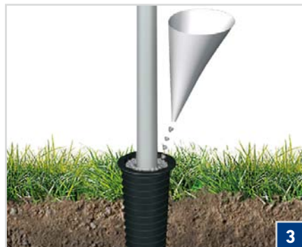
3 Fill special granulate into the screw foundation around the vertical post.
